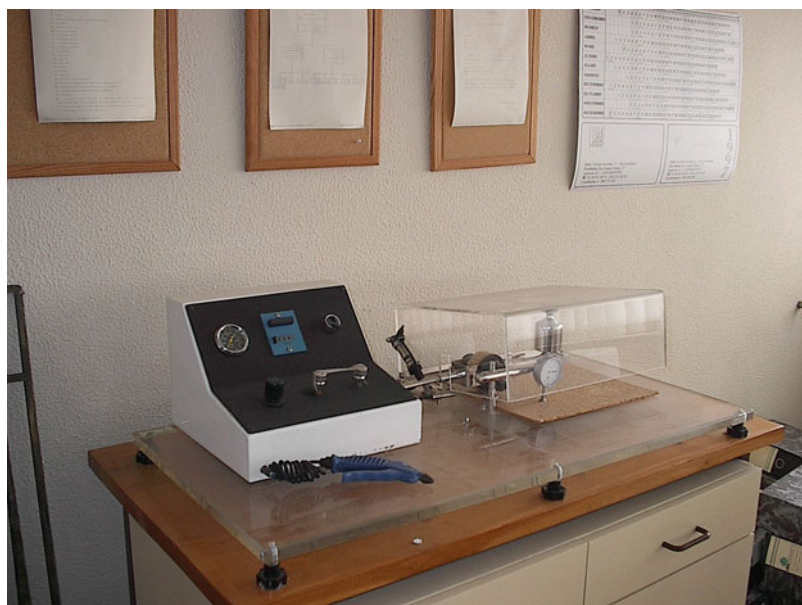
Fig. 13.15 Abrasion test for cork flooring
