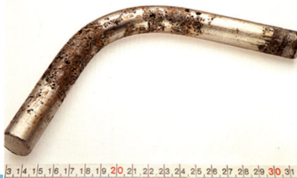
Fig. 15.7 Example of pitting corrosion, in Corrosion Atlas (case 04.06.12.02) [4]
