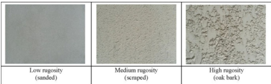
Fig. 2.29 Rugosity of premixed mortar coatings [42]
