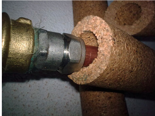
Fig. 13.19 Tubing insulation with extruded agglomerated cork
