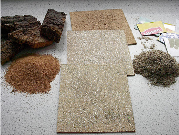
Fig. 13.20 New products based on cork and carton-packaging waste
