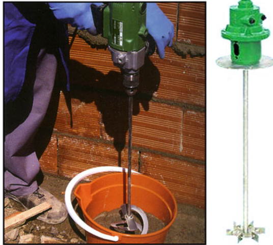
Fig. 3.45 Mixing with an electric mixer [35, 38]
