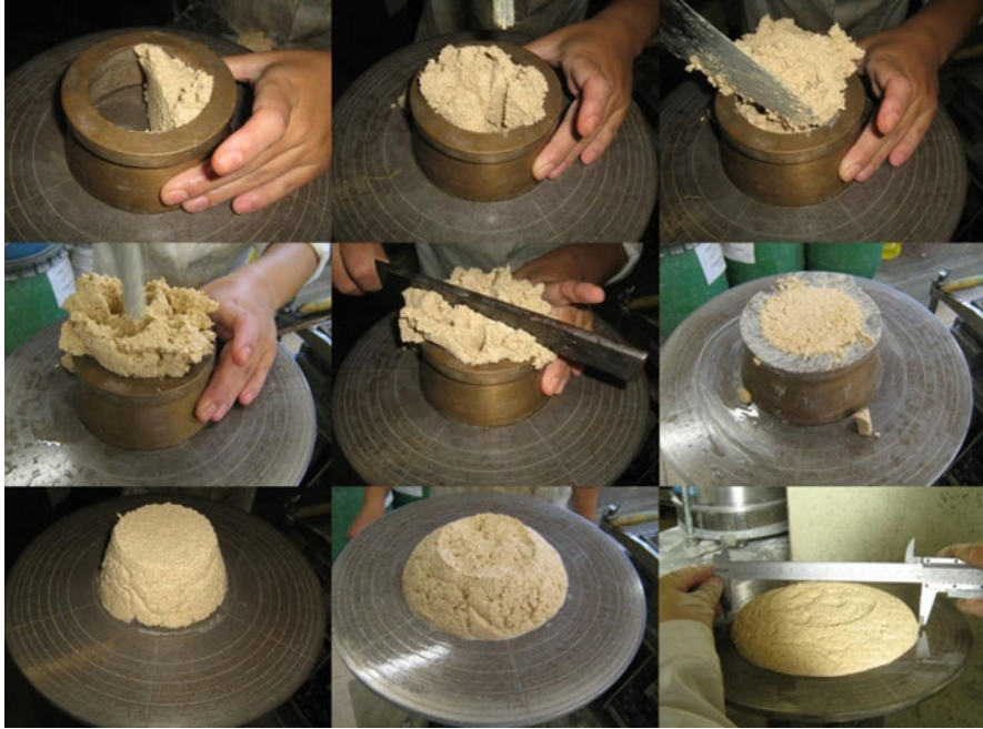
Fig. 2.2 Slump flow test to evaluate the consistency of fresh mortar [30]
