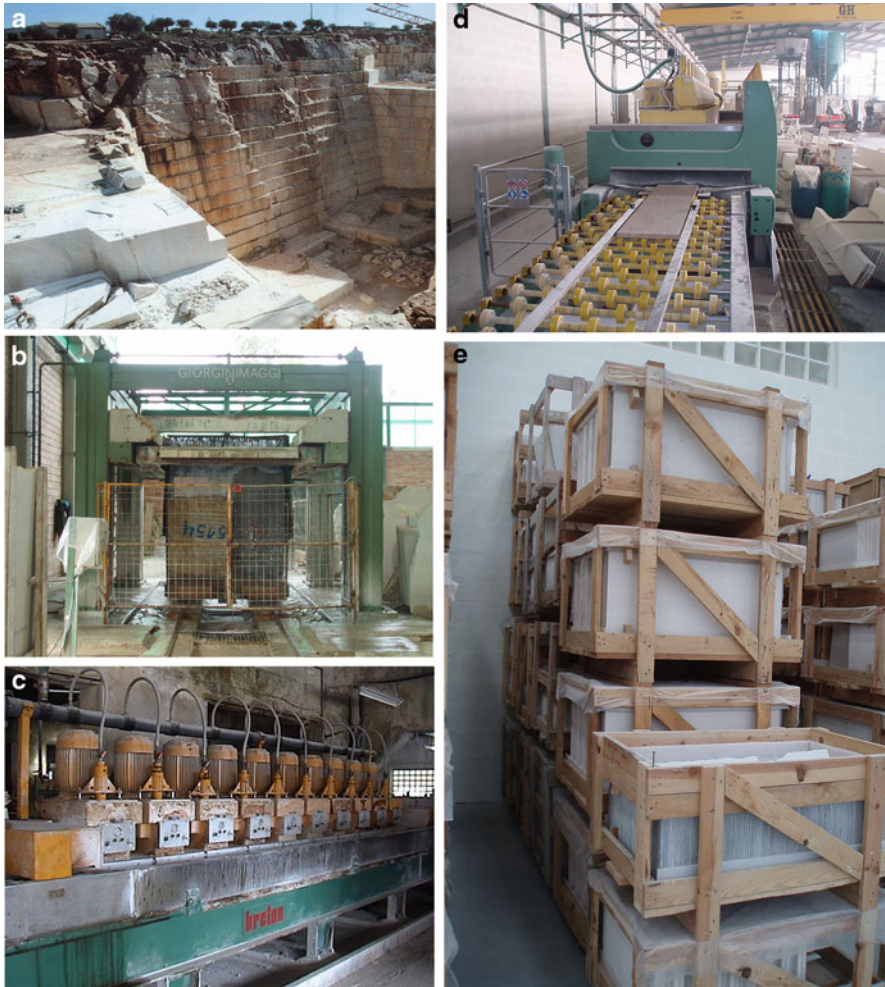
Fig. 9.2 Examples of a common stone production cycle in Portugal: (a) block quarrying, (b) block cutting into slabs, (c) slabs polishing, (d) slabs final cut for smaller slabs or tiles, (e) packing and dispatch
