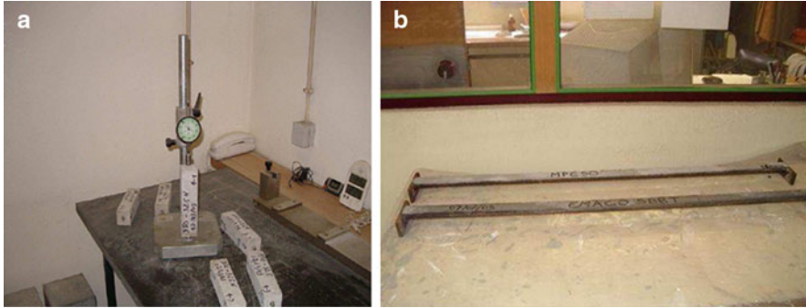
Fig. 2.4 Free shrinkage test with (a) measurement of the relative displacements of the tops; (b) bracket test to evaluate the render's cracking propensity [35]
