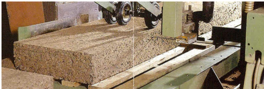
Fig. 13.7 Cutting the block into boards
