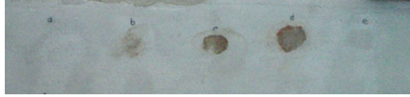
Fig. 3.10 Dirt resistance tests using staining products [13]
