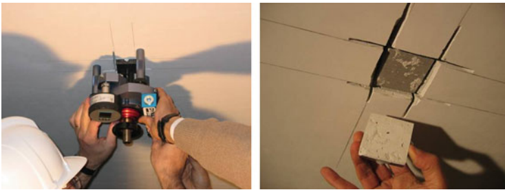
Fig. 3.7 Pull-out test and adhesive failure in the interface between the ceiling's gypsum coating and the concrete substrate
