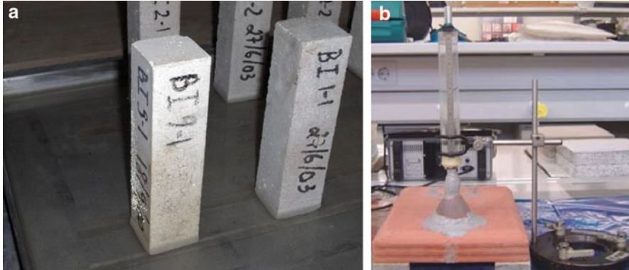
Fig. 2.13 (a) Capillary absorption test on lime mortar specimens [21]; (b) water permeability test [53]
