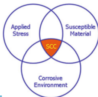
Fig. 15.14 Illustration of the dependence of characteristics in the combination of material/environment/stress in stress corrosion cracking (SCC) and example of SCC in a stainless steel knife (photograph by the author)
