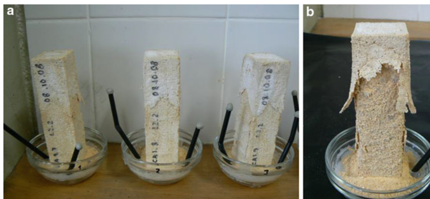
Fig. 2.15 (a) Test by contamination of mortars by capillary rise of a solution of sodium chloride at 15 %; (b) sample at the end of the test [photos by R. Nogueira]
