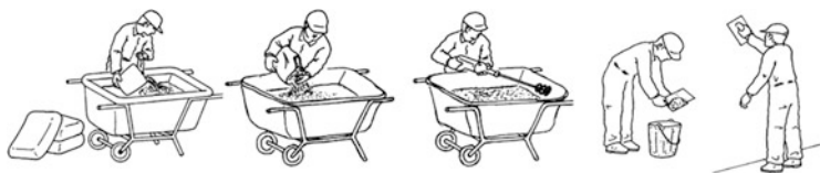
Fig. 3.17 Manual execution procedure of nontraditional gypsum plasters [26]
